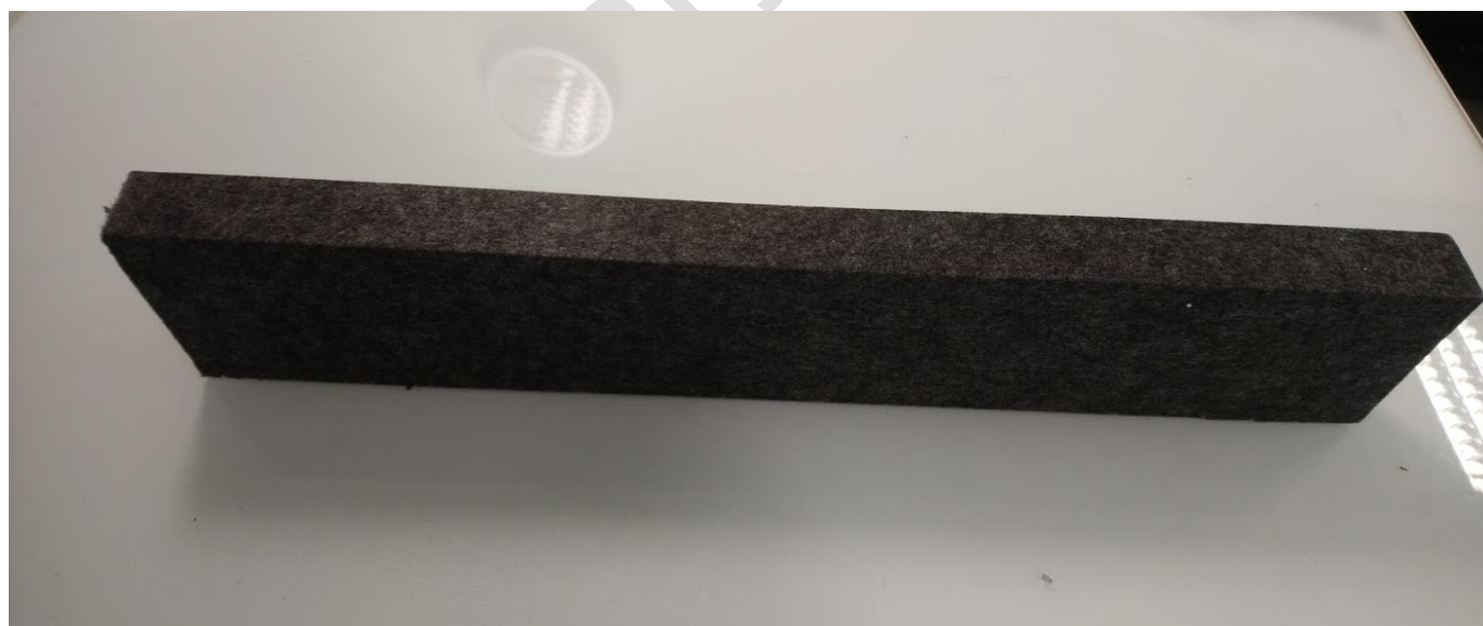
Figure 1 : Test specimen of the ECHOSHAPE Linear Feltline ceiling
